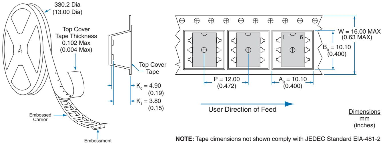
**NOTE:** Tape dimensions not shown comply with JEDEC Standard EIA-481-2
